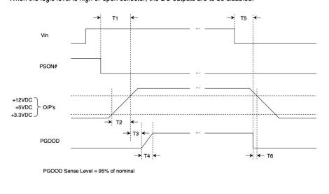
• T1: Power-on time. The time from when PSON# is pulled low to when the +12V, +5V and +3.3V outputs are within the regulation ranges. The power-on time shall be less than 500ms (T1 < 500ms)
